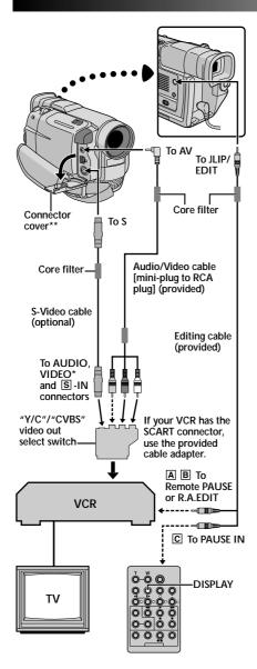
\* Connect when an S-Video cable is not used. \*\* When connecting cables, open this cover.
